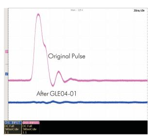
Impulse response of GLE04-01 (into 10 Ohms load)
