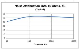
Frequency response of GLE04-01 (into 10 Ohms load)
